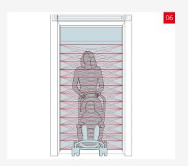
**Multi-Beam Door Sensor (Standard feature)** Multiple infrared light beams cover the door height range of 20mm to 1841mm from the floor level to detect passengers or objects. When any of the beams are blocked, the closing doors immediately reverse to re-open safely without touching the door as providing standard feature.
